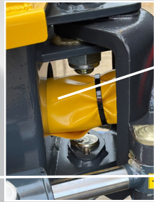
Protected hose lines
