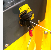
Two stage start inhibitor safety system
