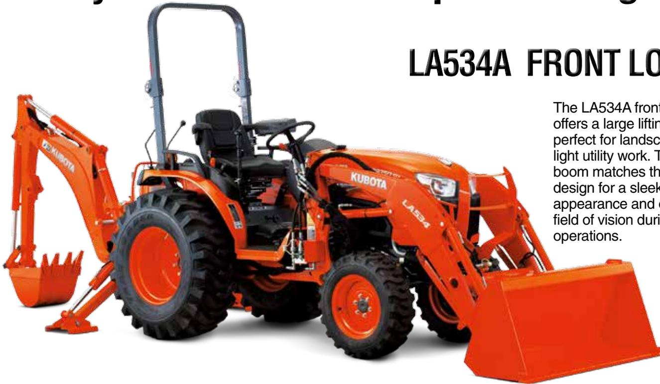
The LA534A front loader offers a large lifting capacity, perfect for landscaping or light utility work. The curved boom matches the new hood design for a sleek and modern appearance and offers a better field of vision during front loader operations.
