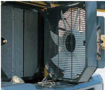
The radiator, air-to-air cooler and oil cooler are mounted side-by-side for more efficient cooling and easy cleaning. A fully-opening, gas spring assisted rear grill gives the operator excellent access to the swing-out fan and coolers.
