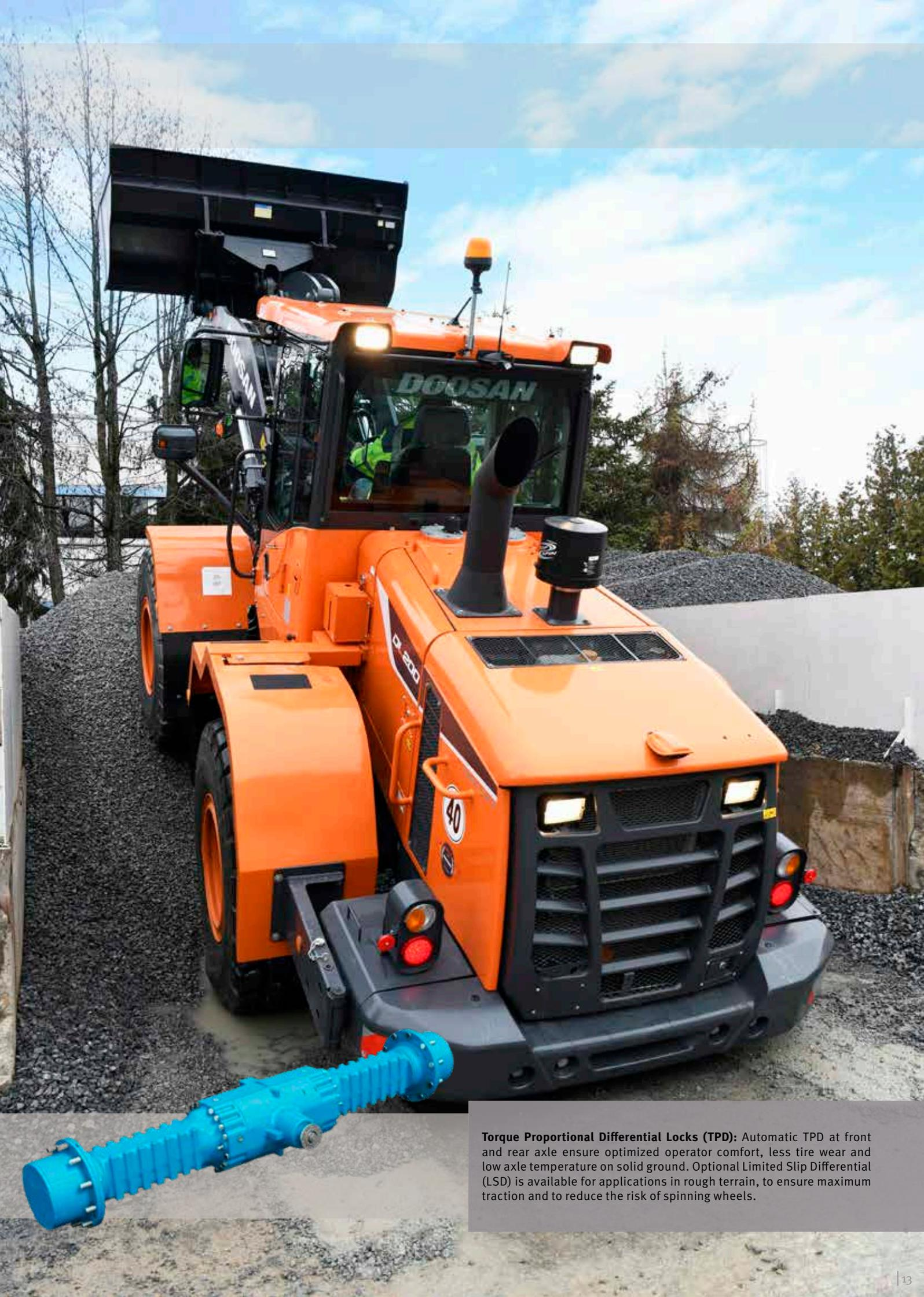
**Torque Proportional Differential Locks (TPD):** Automatic TPD at front and rear axle ensure optimized operator comfort, less tire wear and low axle temperature on solid ground. Optional Limited Slip Differential (LSD) is available for applications in rough terrain, to ensure maximum traction and to reduce the risk of spinning wheels.
