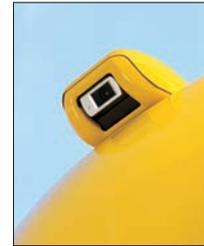
The operator can view the rear of the machine with a color monitor screen.
